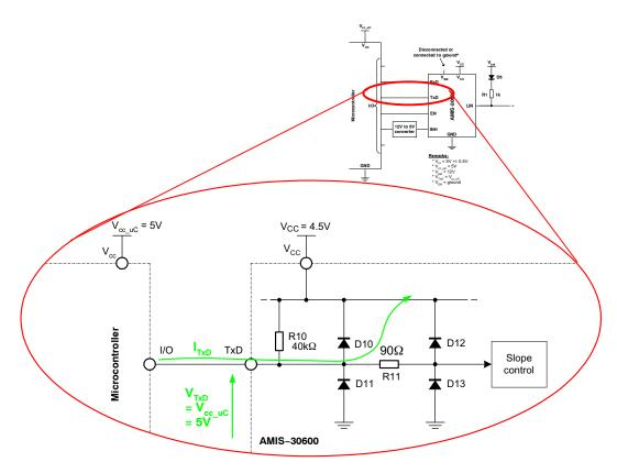
Figure 8. ESD Protection Diode D10 and/or D12 Conducts<sup>5</sup>
