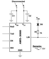
Figure 16. Decoupling Capacitor Present when V<sub>BB</sub> and V<sub>CC</sub> Disconnected
