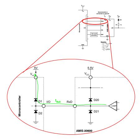
Figure 10. ESD Protection Diode D1 Conducts<sup>8</sup>
