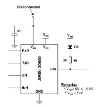
Figure 12. Decoupling Capacitor Present when V<sub>BB</sub> is Disconnected
