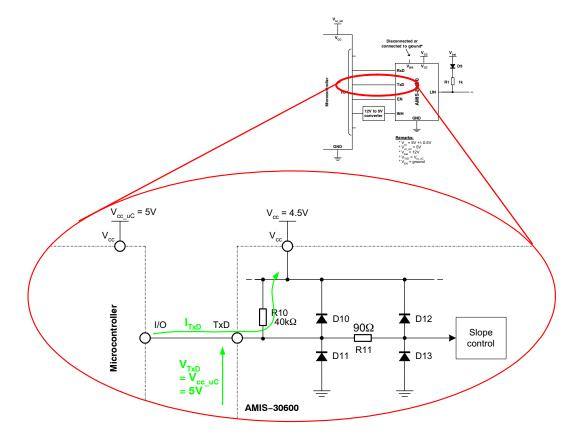
Figure 9.  $I_{TXD}$  when ESD Protection Diodes Don't Conduct^7
