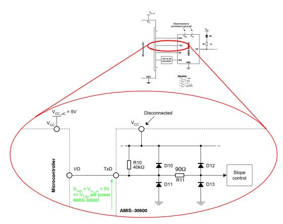
Figure 14.  $V_{TxD}$  will Power AMIS-30600 when  $V_{CC}$  is Disconnected<sup>11</sup>
