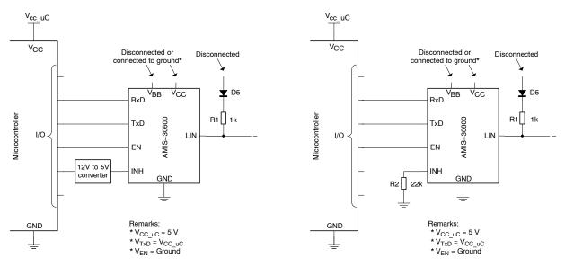
Figure 3. LIN Pullup Resistor Disconnected
