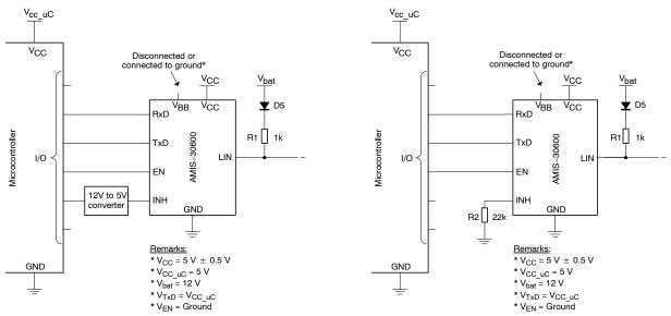
Figure 1.  $V_{\mbox{\scriptsize BB}}$  Disconnected or Connected to Ground
