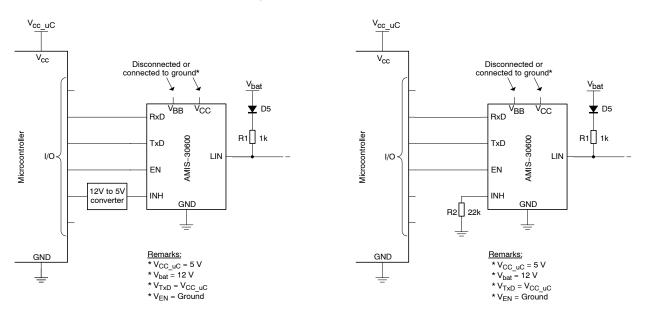
Figure 2. V<sub>BB</sub> Disconnected or Connected to Ground
