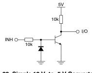
Figure 22. Simple 12 V-to-5 V Converter with Comparator
