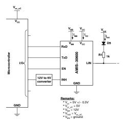
Figure 11. Current Consumption First Setup
